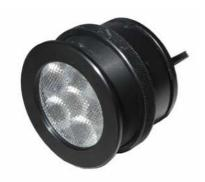
Panel System LED lighting. Anodized aluminum illuminator with 6 power LED sources and 8°-25°-40° lens. Threaded ring for fastening. Separated external PSU.
